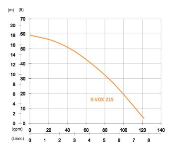
Shaft Speed: 2850 rpm Outlet: 50mm, 2in
